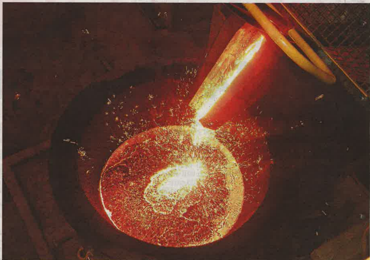
A ferrovanadium pour at Atlantic's Windimurra operations.
